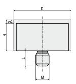
A pressure housing is a method of protecting a magnet from high pressure or aggressive media. This is made from robust stainless steel and resists pressures up to 400 bar.
