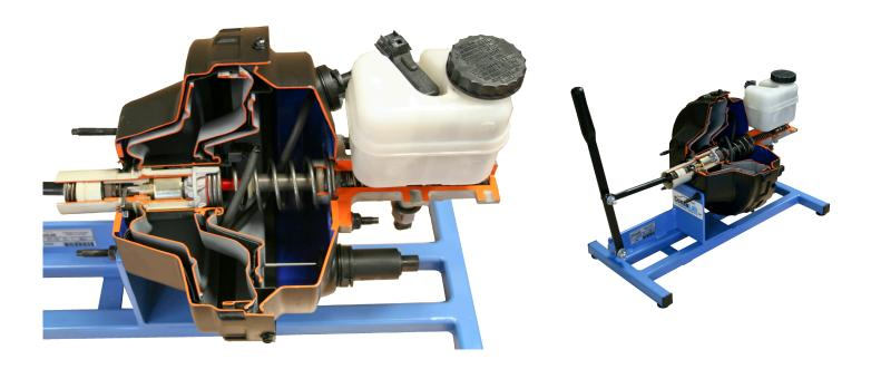
The ConsuLab EC-122 cutaway allows to visually demonstrate the operation and internal parts of a vacuum brake booster and master cylinder. The trainer is equipped with a braking handle that simulates the brake pedal for educational purposes. On a vehicle when the driver depresses the brake pedal, the movement is transformed into hydraulic pressure that is delivered to hydraulic cylinders at the four wheels through pipes and hoses using an incompressible fluid.
