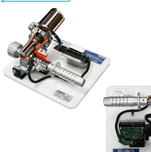
The ConsuLab EC-140-15 Cutaway Electric Assist Power Steering, allows the student to understand the basics of an electric assist power steering as used in today's vehicles. It has two handles representing the steering wheel and steering column.
