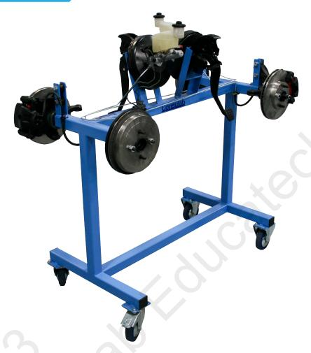
The EM-123 2D double-sided two-wheel hydraulic brake system trainer is used to demonstrate the functionality of a typical hydraulic braking system as it operates on a real vehicle. The trainer is built with OEM components and is based on the Toyota Yaris non-ABS platform. This space saving double work station can be used in the classroom environment for demonstrations to students.
