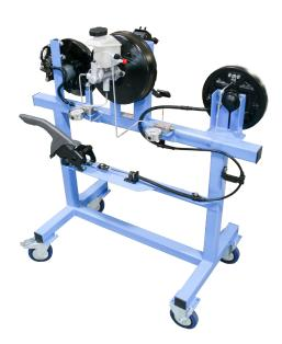
The EM-123 Two-wheel hydraulic brake system trainer is used to demonstrate the functionality of a typical non-ABS braking system as it operates on a real vehicle. The trainer is built with OEM components and is based on the 2011 Kia Rio platform. The trainer can be used in the class-room environment for demonstrations to students. The trainer provides a safe and effective method of demonstrating the principles of hydraulic braking systems used on today's vehicles.
