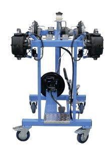
The EM-123-4 CIVIC 4-wheel hydraulic brake system trainer is used to demonstrate the functionality of a typical non-ABS braking system as it operates on a real vehicle. The trainer is built with OEM components and is based on the 2007-2010 Honda Civic platform. The trainer can be used in the classroom environment for demonstrations to students. The trainer provides a safe and effective method of demonstrating the principles of hydraulic braking systems used on today's vehicles.
