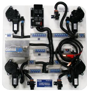
The EM-200-02D4 Four-door Power Window System Trainer allows for the demonstration of a complete power window system using real-world components. Terminal block receptacles are provided for diagnostic test points.
