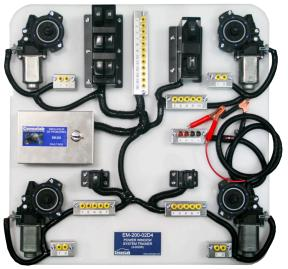
The ConsuLab EM-200-02D4 is a functional Power Window System Trainer mounted on a plastic training board with the following features:
