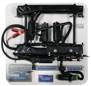
The EM-200-05 trainer allows for the demonstration of a complete power seat system using real-world components. Terminal block receptacles are provided for diagnostic test points.
