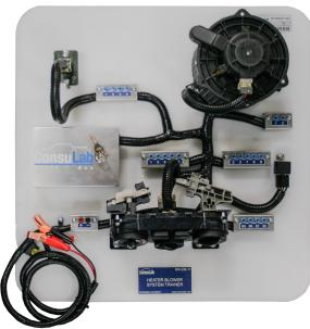
The ConsuLab EM-200-11 trainer allows for the demonstration of a complete blower motor system using real-world components. Terminal block receptacles are provided for diagnostic test points.
