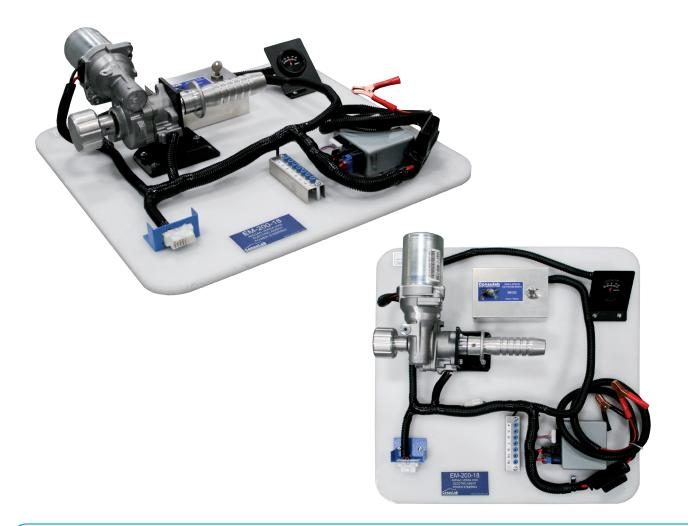
The EM-200-18 is a fully functional electric power steering trainer. The trainer provides a safe and effective method of demonstrating the principles of electric power steering systems used on today's vehicles. It is based on a 2007 and newer Nissan Versa vehicle but other common vehicles also use this system design.
