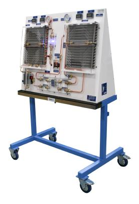
The ConsuLab EM-2000-HB Air Conditioning trainer is a complete A/C system with unique features designed to enhance the instruction of air conditioning physics. The trainer uses the H-Block TXV design of refrigerant flow control. The trainer uses common automotive components and can be used in both classroom and shop environments. The trainer utilizes a hermetically sealed and internally protected compressor. Operates on 120V 15A 60Hz circuit.
