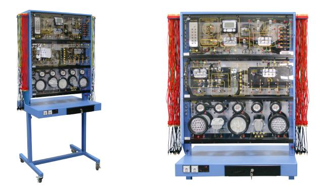
The ConsuLab MP-1918-1D is a double-sided CAN Bus Multiplex trainer that communicates in J-1939 protocol. Digital and analog inputs and outputs can be activated. Analog signals can be displayed using the J-1939 display. The trainer utilizes the "Moduponent<sup>™</sup>" design feature which allows unlimited expansion capabilities. This unit is equipped with an integrated electronic fault box containing 12 faults on each side.
