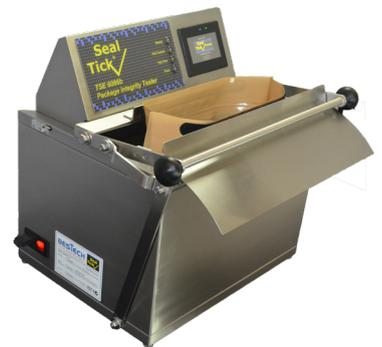
**TSE6086b in open position, ready for next package to be loaded**
