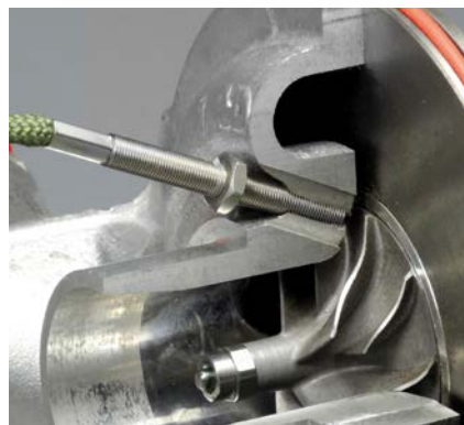
Large measuring distances both at aluminium and titanium
