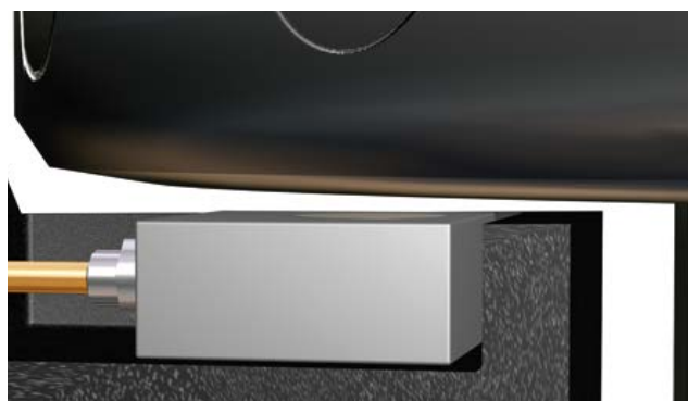
Measuring the thermal extension
