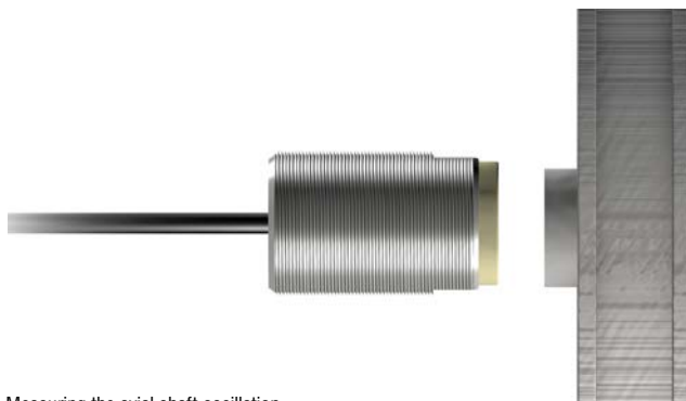
Measuring the axial shaft oscillation
