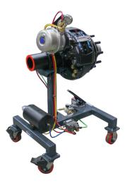
The ConsuLab HV-126-DISC trainer includes a heavy duty truck disc assembly with air chamber. Using shop air; the service and parking brakes can be applied, the brake system can be dismantled, adjusted and the brakes can be measured. The trainer includes a sectional cutaway showing bearings, bearing races and caliper assembly.
