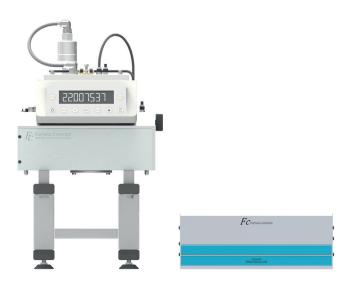
For increased ease-of-use the control box can be used to set the desired pressure between the test and reference ports (differential mode) or the test port and atmospheric pressure (gauge mode) of the FRS4 instrument.
