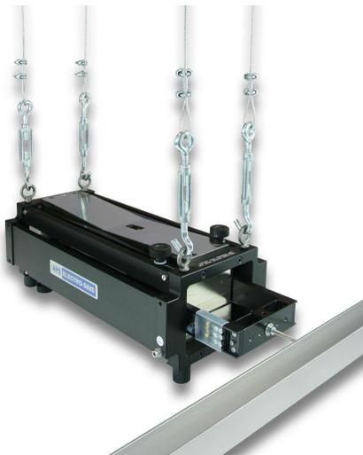
APS 113 with APS 8610 - Modal Stinger and APS 8611 - Steel Cable Kit prepared for Free Body Mode operation
