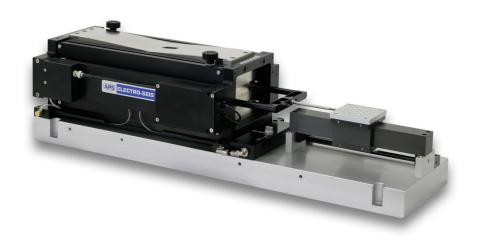
The **APS 500 ELECTRO-SEIS**<sup>®</sup> Air Bearing shaker is a long stroke, electrodynamic force generator specifically designed to be used for calibration and evaluation of position and acceleration sensors or other motion transducers. It provides excellent properties for low frequency excitation of such devices. The model consists of an air bearing driver attached to an air bearing load mounting table that allows payloads up to 3.0 kg (6.6 lb).
