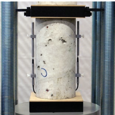
Measuring Range: 1, 2.5, 5 or 10 mm Fixtures clued onto the sample.
