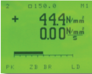
Testing of Cubes Example: Determination of the Compressive Strength of Cubes 150 mm.
