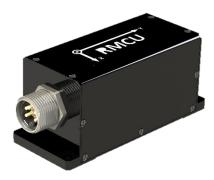
The Inertial Labs **RMCU** utilizes 3-axes each of precision MEMS accelerometers, miniature Fluxgate magnetometers and MEMS gyroscopes to provide accurate Heading, Pitch and Roll of the device under measure. Integration of gyroscopes' output provides high frequency, real-time measurement of the device rotation about all three rotational axes.
