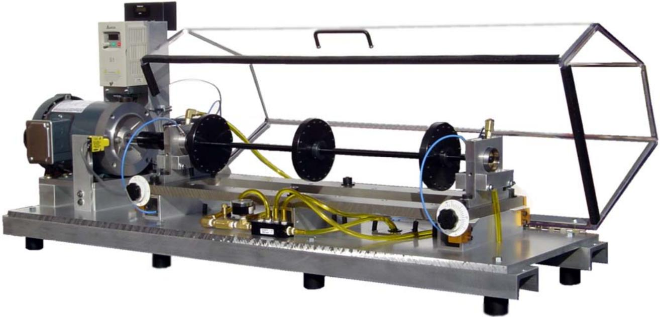
Spectra Quest's Machinery Fault & Rotor Dynamics Simulator (MFS-RDS) is an innovative tool to study the dynamic behavior for rotor supported by oil lubricated journal bearings, as well as other common machinery faults, such as balancing and resonance study. An oil pump is provided with the simulator to drive the lubrication fluid. In addition, it provides different bearing clearance selection and controllable lubrication oil pressure for rotor dynamics whirl and whip phenomena.
