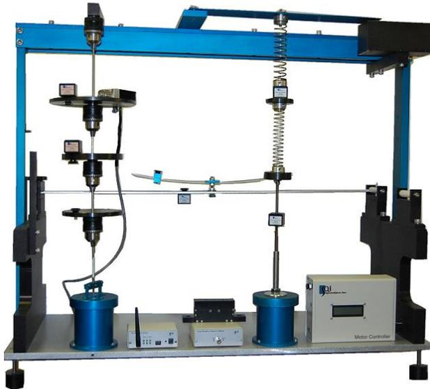
The Vibration Fundamentals Training System (alias VFT) is a turn-key integrated educational package for teaching/learning the fundamental principles of mechanical vibration as well as engineering mechanics. It provides both a comprehensive hands-on experimental device and an instrumentation package including **wireless sensors** for performing laboratory exercises to enhance student understanding of vibration theory.
