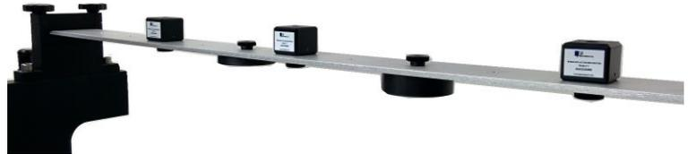
**Includes:** Three different beams (aluminum, steel, and plastic), mode shape animation software and shaker frequency sweep software for excitation of different modes, and three masses.
