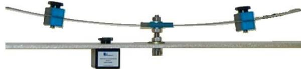
**Includes:** Hardware and software for Tuned-Mass-Damper, one constraint layer and without constraint layer Viscoelastic beams, and two viscous damping setups-one for linear and one for torsional vibration control.
