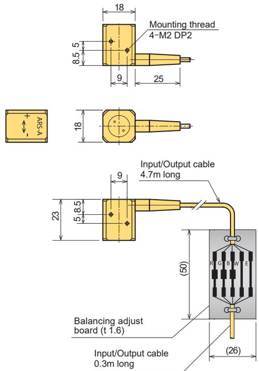
Input/Output cable :  $\phi 3.2\text{mm}$  0.08mm<sup>2</sup> 4-core shielded vinyl cable 5m
