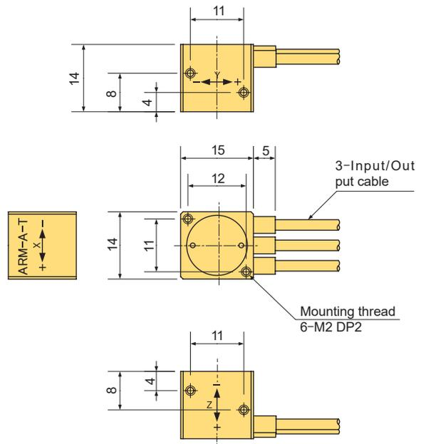
Input/Output cable :  $\phi 2.2\text{mm}$  0.05mm<sup>2</sup> 4-core shielded vinyl cable 5m
