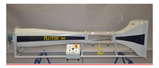
FLOTEK® 360 is a small benchtop wind tunnel made for classrooms where space and transport are a primary concern. This low noise classroom wind tunnel can be mounted to a bench or you can utilize an optional mobile stand to move the wind tunnel to different locations. This entry level wind tunnel is great for smaller middle schools, high schools, and technical colleges.
