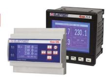
The Exa series are microprocessor-based energy meters / analyzers suitable for harsh environments. Equipped with an RS485 Modbus RTU port. Indication of the phase sequence, four operating time counters in addition to more than one hundred measurements. Versions with digital and analogue inputs - outputs. Perform the functions of analyzer, counter and multimeter.
