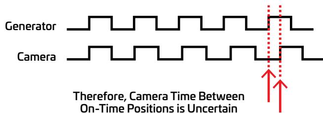
The common approach used by most high-speed camera manufacturers is that the camera timing is allowed to drift and only re-set at each on-time position. Therefore, at the end of each one-second time period there could be a substantial error. This is compounded if the IRIG signal is lost and the signal drifts.
