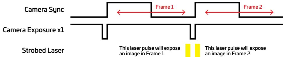
**Two exposures in a single frame:** Currently if a user is trying to understand the motion of a bullet, they increase the frame speed of the high-speed camera to see enough frames of motion; increasing frame rate has the effect of decreasing
