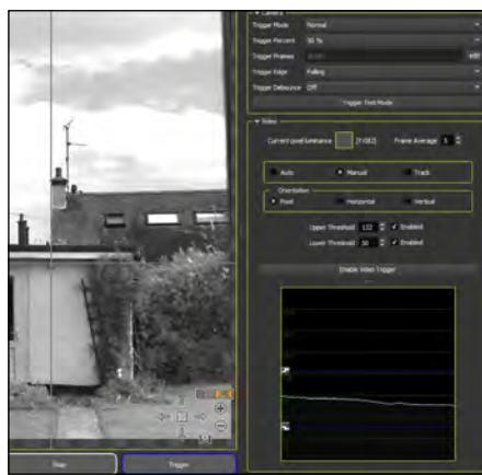
Manual mode provides more control than Auto. For example, the user may only want to run with an upper threshold (trigger on brighter, not darker).
