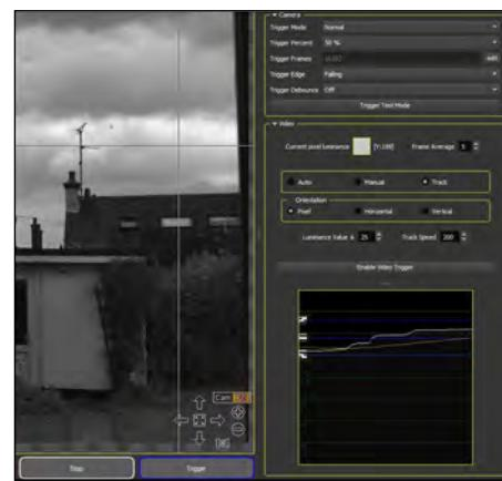
The Track mode allows the luminance to change slowly without triggering the camera, and only allows a trigger to occur when the luminance changes quickly. An example for use is in an outdoor environment with cloud cover where the ambient brightness will vary slowly.
