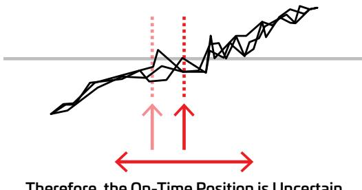
Some IRIG generators produce a jittery signal—digital sampling adds to this. Therefore, the on-time position is uncertain.
