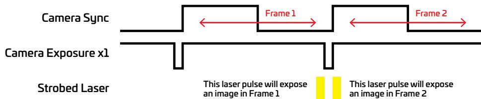
**Two exposures in a single frame:** Currently if a user is trying to understand the motion of a bullet, they increase the frame speed of the high-speed camera to see enough frames of motion; increasing frame rate has the effect of decreasing the resolution.
