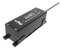
The Inertial Labs AHRS-I utilizes 3-axes each of precision accelerometers, magnetometers gyroscopes to provide accurate Heading, Pitch and Roll of the device under measure. Integration of gyroscopes' output provides high frequency, real-time measurement of the device rotation about all three rotational axes. Accelerometers and magnetometer measure absolute Pitch, Roll and magnetic Azimuth at AHRS initial alignment as well as providing ongoing corrections to gyroscopes during operation.
