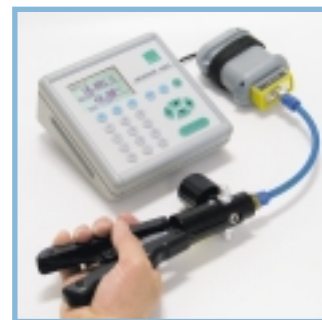
Pressure generation with hand pump
