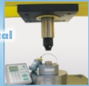
Force calibration of a press
