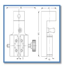
Shown above the grip with a preset face on one side and a adjustable T-bar on the other, the grip carrier plate and the plain and diamond faces. The outline drawing shown for reference only
