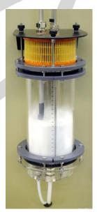
the surface temperature, and the other, in conjunction with a controller, prevents the heater surface temperature exceeding a set value (up to  $200^{\circ}$ C). A digital temperature indicator with a selector displays the temperatures of the element, the air supplied to the distributor, and the moveable probe in the bed chamber.
