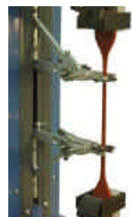
Extensometer arms closed and engaged with sample
