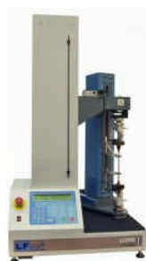
EX250Plus fitted to single column test machine
