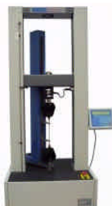
EX800Plus fitted to twin column test machine
