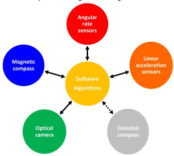
Each of the technologies compensate for each other's deficiencies and errors, acting as a self checking and calibrating system. For example, if a magnetic change is sensed, but the camera and accelerometers see no change - the magnetic change is ignored.
