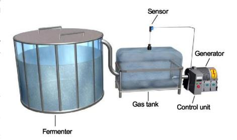
The distance between film and displacement sensor increases as the filling quantity in the gas tank decreases.
