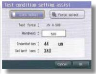
In standard test mode, test can be performed by setting detailed conditions such as sample information, shape corrections, and pass/fail determinations. Fracture toughness tests are also possible. Simple test mode can be selected to start testing immediately just by setting the test force and the duration time.
