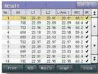
Test results can be listed and statistics cam be displayed. Results can be written in text format to a USB memory stick.
