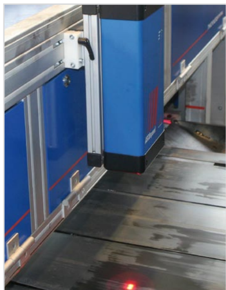
Picture: ASCOSpeed for strip length measurement
