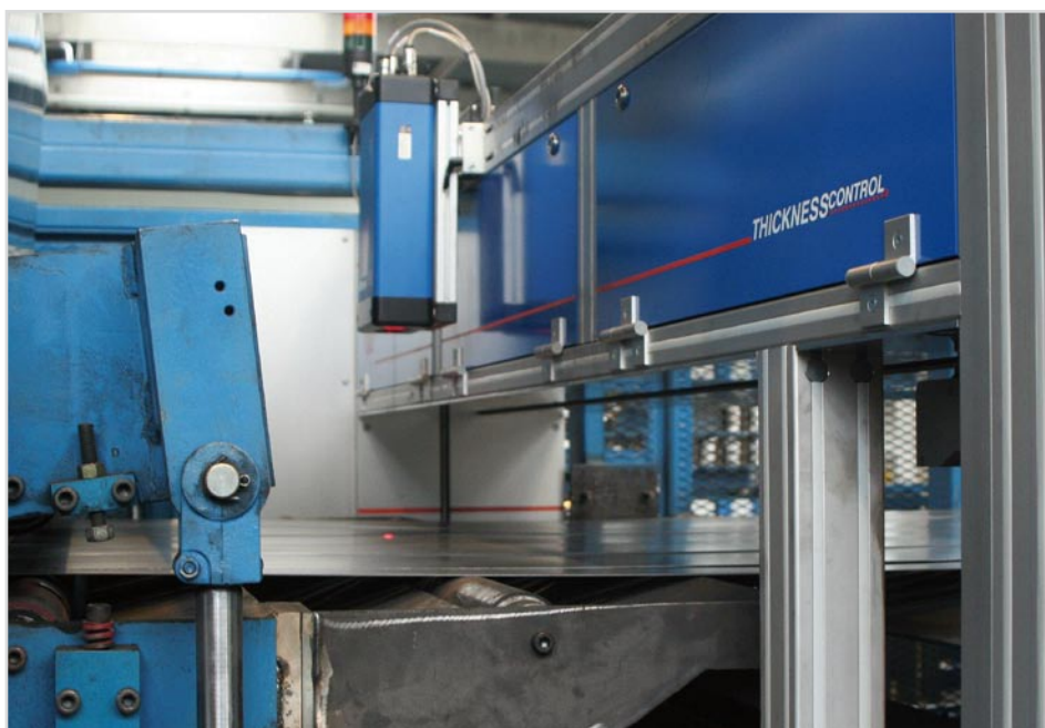
Picture: Installation O-frame with ASCOSpeed in a cutting line
